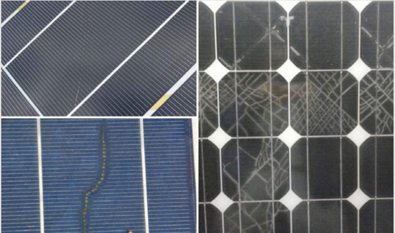
Fig 1: damage due to manufacturing, transportation/installation and the environment
