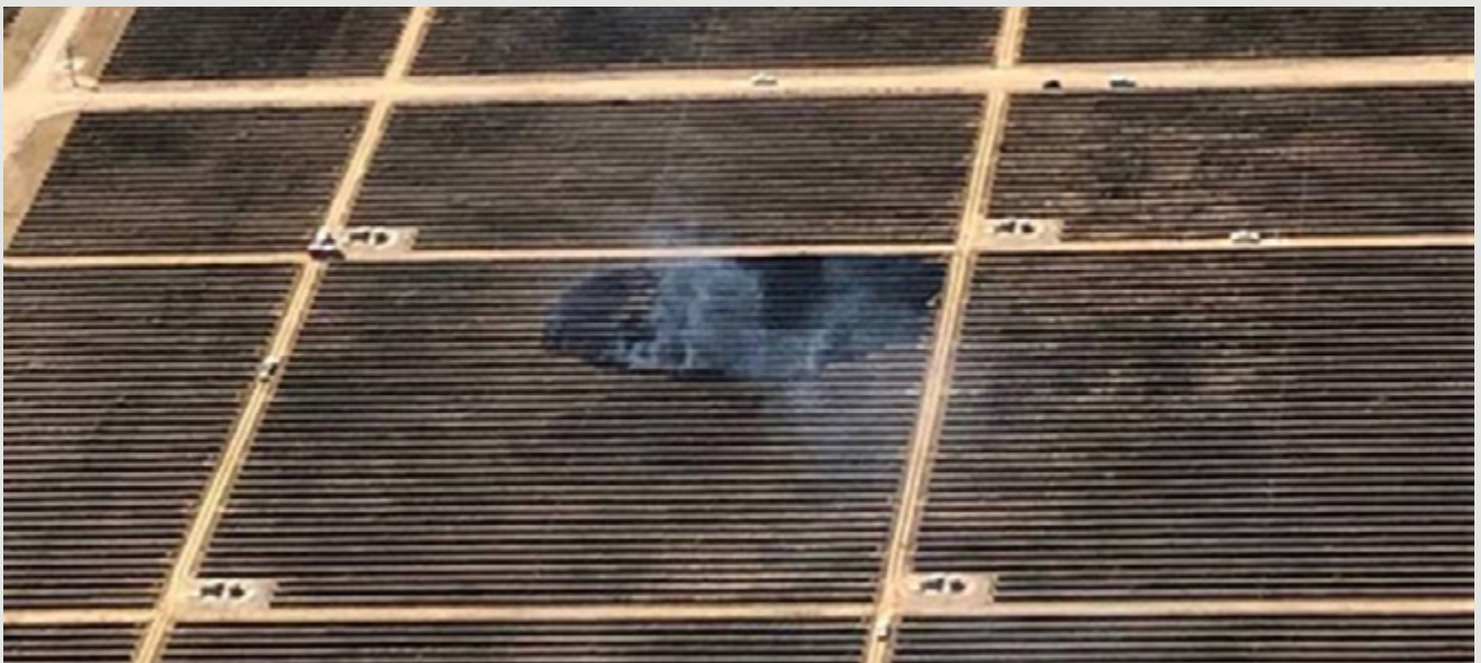
Fig 1: A 2020 on-site vegetation fire, under a California solar array; this fire spread from two acres when reported to six acres before controlled by the local fire department.
